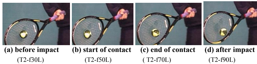
Figure 1 Topspin impact of a tester in this experiment.
