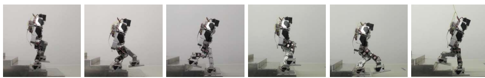
Fig.12 Six states of GENBE-No.4 with 10 freedom legs for going down the stairs with instability
