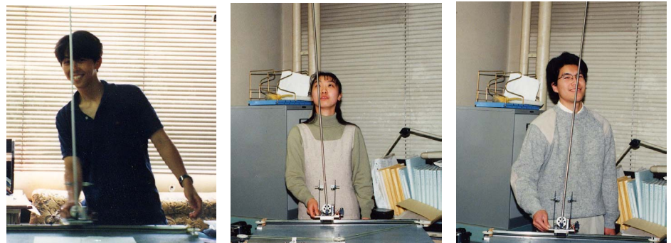
Fig.1 Stabilizing control of an inverted pendulum.
