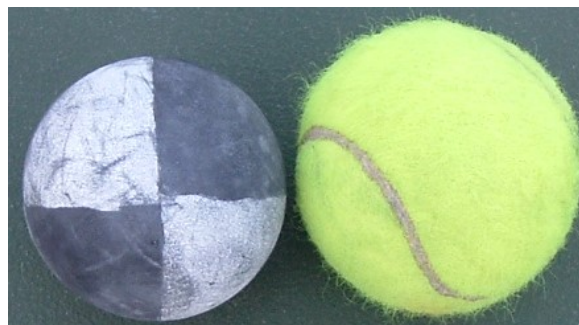
Fig.9 Tennis ball (right) and a smooth surface ball without felt (left).
