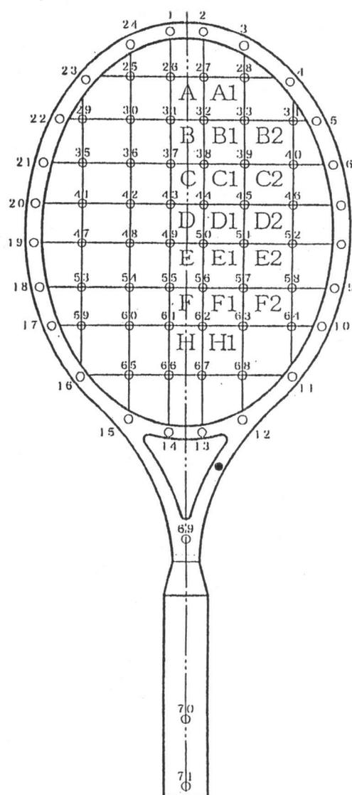
Fig. 2 The impact locations between a ball and a racket, where the shock vibrations be predicted.
