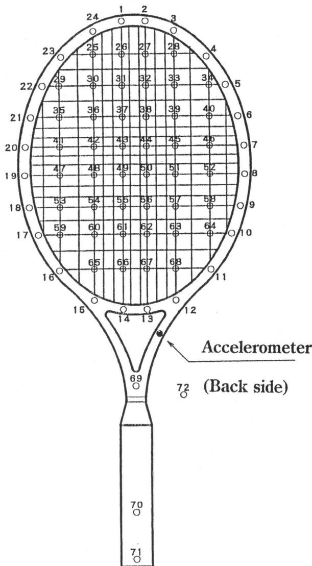
Fig. 1 The impact points of a racket using hammering method for identification of vibration characteristics.
