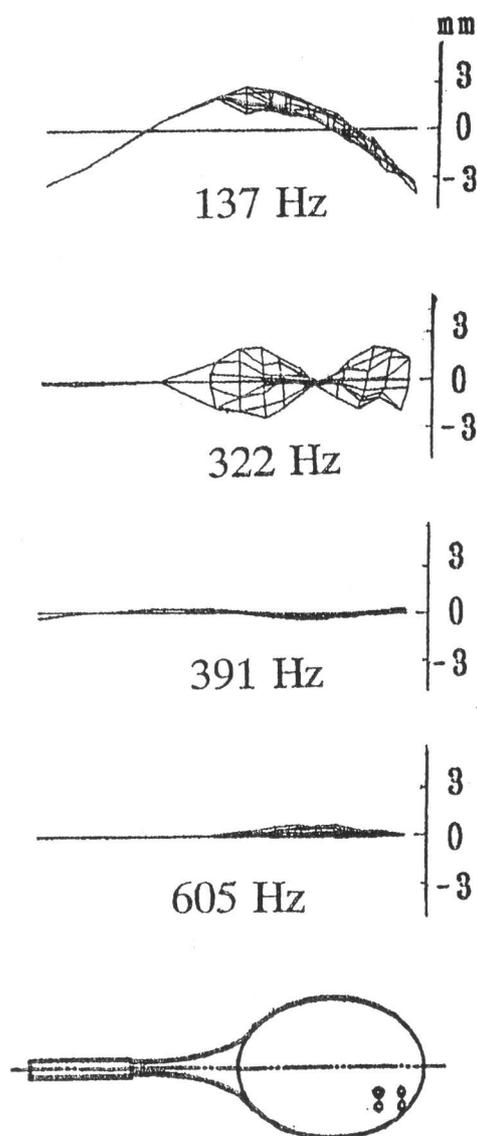
Fig.3 Example of predicted initial amplitude components of racket vibrations when a ball strikes off-center of a racket face (Impact location B2).
