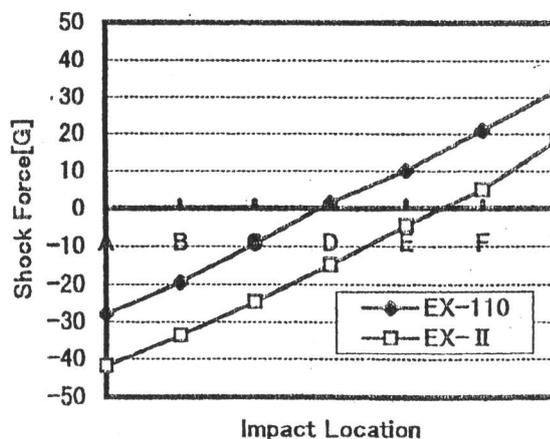
Fig.5 Predicted maximum shock acceleration at the grip (70 mm from grip end) with an equivalent mass of an arm vs. impact location (Impact velocity:30 m/s).
