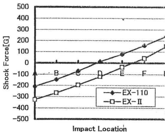
Fig.4 Predicted maximum shock acceleration at the grip (70 mm from grip end) of freely-suspended racket vs. impact location (Impact velocity: 30 m/s, EX-II:100 in<sup>2</sup>, EX-110:110 in<sup>2</sup>)
