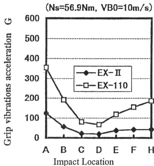
Fig.6 Summation of the predicted grip acceleration amplitude considering four vibration mode components when a player hits flat forehand drive, where a simple swing model is used (Racket EX-II:100 in<sup>2</sup>, EX-110:110 in<sup>2</sup>).
