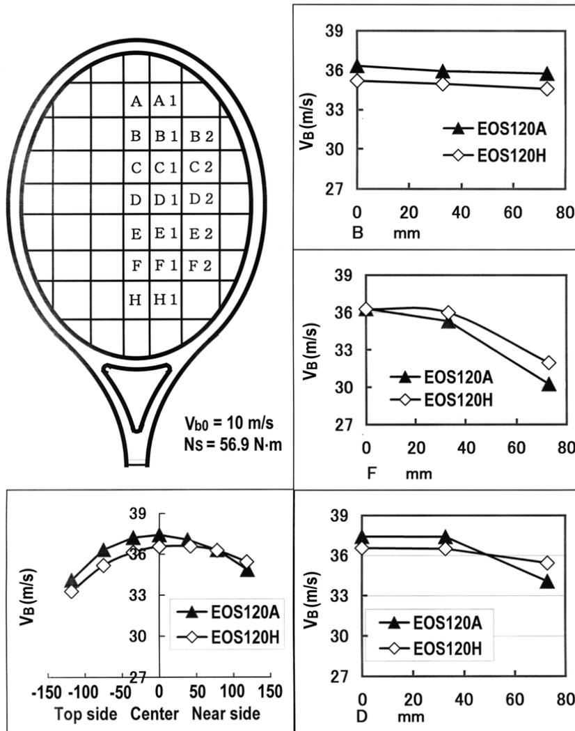
Fig.6 Predicted post-impact ball velocity  $V_B$  when a player hits the ball at the longitudinal axis and off the longitudinal axis ( $V_{Bo} = 10 \text{ m/s}$ ,  $N_s = 56.9 \text{ Nm}$ ).
