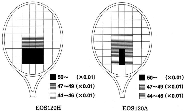
Fig.4 Sweet area with respect to the rebound power coefficient  $e$  ( $V_{Bo} = 10$  m/s,  $N_s = 56.9$  Nm).
