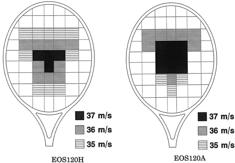
Fig.7 Predicted sweet area with respect to the post-impact ball velocity  $V_B$  ( $V_{Bo} = 10$  m/s,  $N_s = 56.9$  Nm ).
