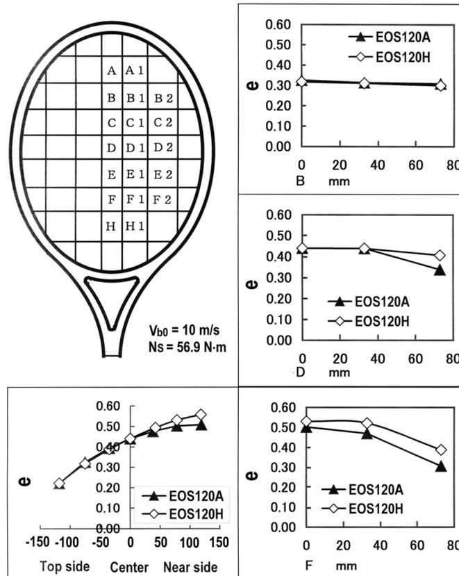
Fig.3 predicted rebound power coefficient  $e$  when a player hits the ball at the longitudinal axis and off the longitudinal axis ( $V_{Bo} = 10 \text{ m/s}$ ,  $N_s = 56.9 \text{ Nm}$ ).
