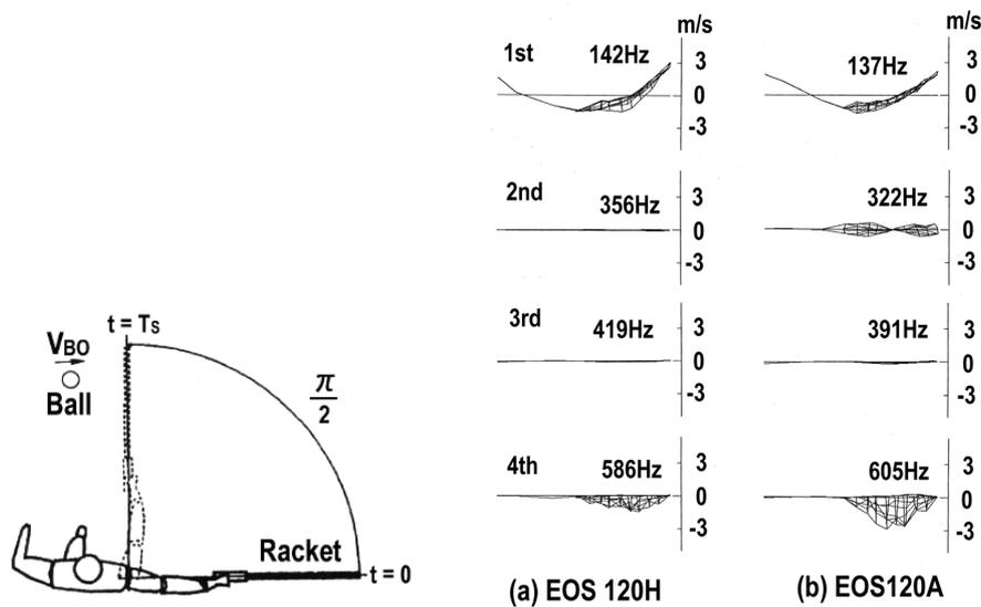
Fig.1 Simple forehand ground stroke swing model.
