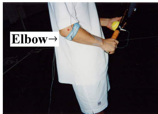
Fig.4 Location of accelerometers at the elbow joint and the racket handle in the service stroke.
