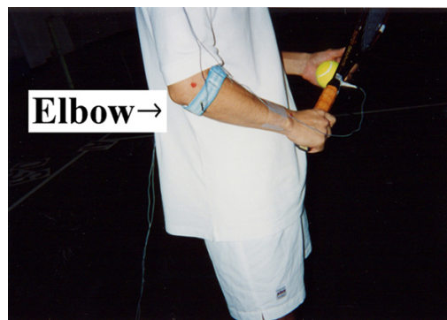
Fig.1 Location of accelerometers at the elbow joint and the racket handle in the service stroke.
