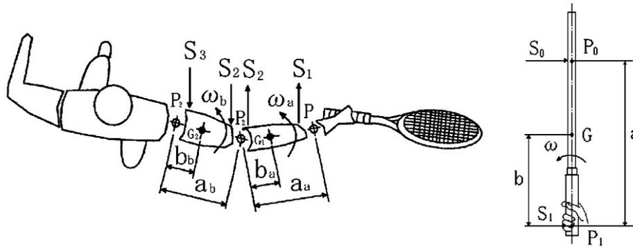
**Fig.1 Impact model for the prediction of the shock force transmitted to the arm joints from a racket.**
