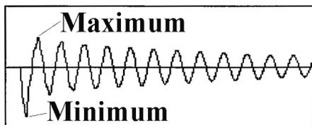
Fig.5 Peak- peak value of the wave form.
