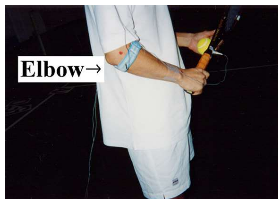
Fig.4 Location of accelerometers at the elbow joint and the racket handle for the service stroke.
