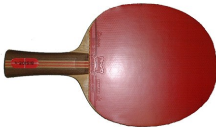
Fig.12 Tested racket BISIDE with rubber SRIVER (1.9 mm sponge).
