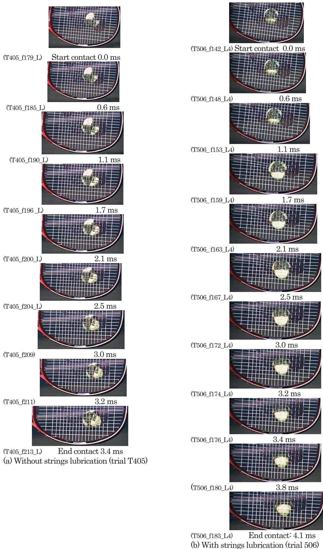
Fig.4 Effect of strings lubrication on the ball spin behaviors (impact views from back side direction with frames per 10^{-4} s). (a) Without strings lubrication (b) With strings lubrication
