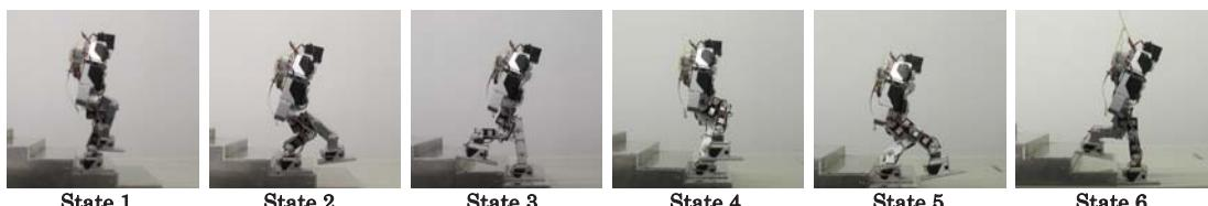
Fig.21 Six states of GENBE-No.4 with 10 freedom legs for going down the stairs with instability
