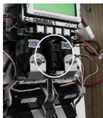
Fig.10 PSD-Sensor of autonomous humanoid biped robot GENBE No.5-2005
