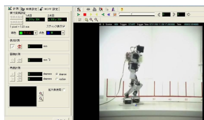
Fig.15 Measurement of Stride vs. Operating Time Setting of Servomotors.
