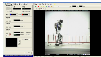
Fig.14 Measurement of Forward Leaning Angle vs. Operating Time Setting of Servomotors.
