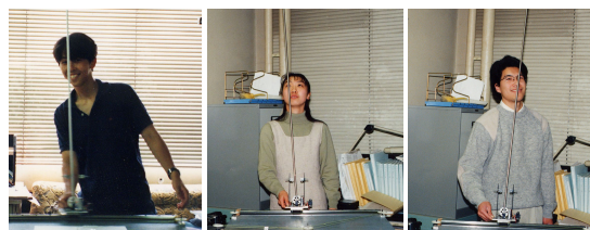
Fig.1 Stabilizing control of an inverted pendulum on a cart by a human operator.
