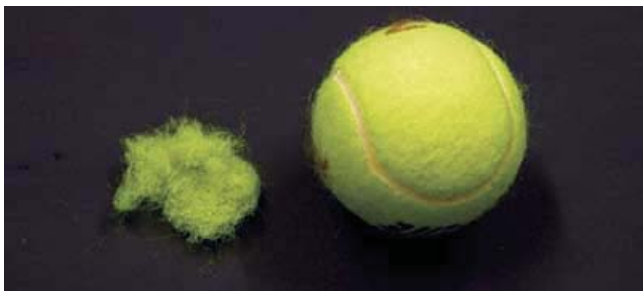
Fig.11 A ball next to 0.22 grams of fuzz. Some balls lost four to five times that much fuzz. (Courtesy of Rod Cross and Crawford Lindsey (3) )
