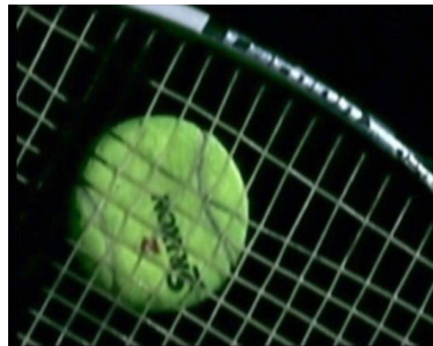
Fig.9 Ball spin behavior and the mechanism for increasing the spin rate in which strings stretch, slide laterally, and spring back the main strings at the string intersections when a ball is released from the string bed for the case of new gut.
