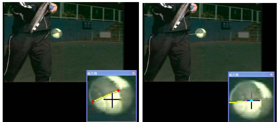
(a) Analysis of spin rate (b) Analysis of ball velocity Fig.8 View of impact and spin behavior analysis.
