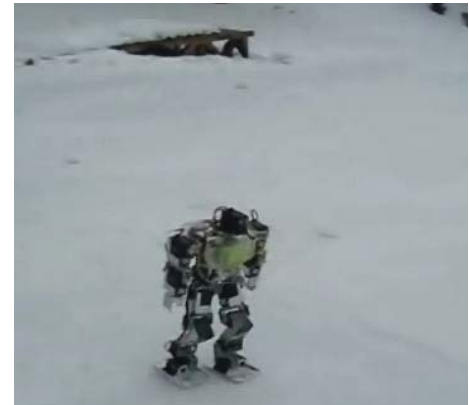
Fig. 29. Robustness of humanoid biped robot Genbe running on ice and snow and taking 9 steps in 1.50 seconds.
