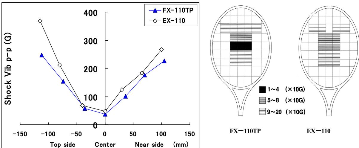
(b) Shock vibrations peak value at the wrist vs. impact locations (Impact velocity : 30m/s)
