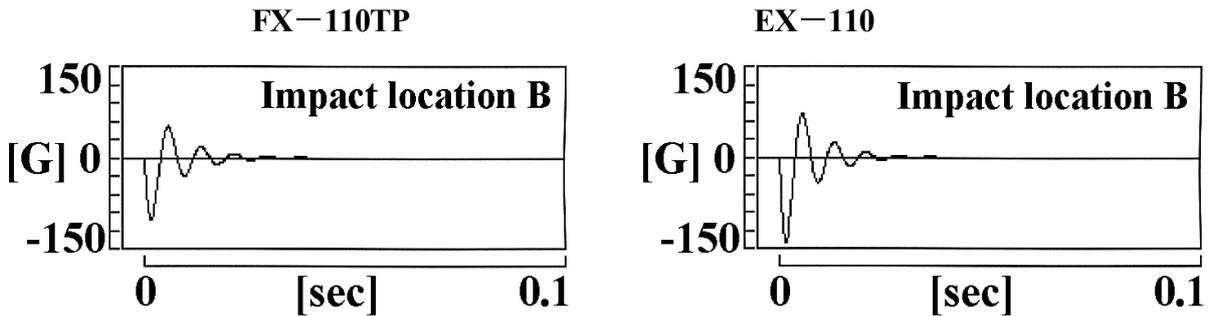
(a) Predicted shock vibrations at the wrist joint (Impact location : Top side B)
