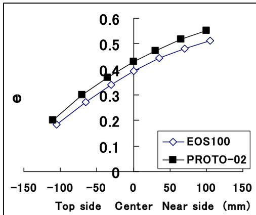
Fig.17 Predicted rebound power coefficient  $e$  ( $N_s=56.9$  Nm,  $V_{Bo}=10$ m/s)
