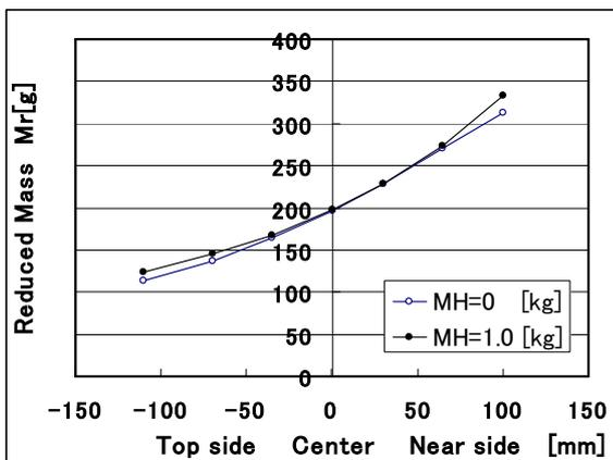
Fig.8 The effect of the arm on the reduced mass of a racket at the impact locations (conventional balanced racket 370 g,  $M_H=1.0$  kg: with arm,  $M_H=0$  kg: without arm)
