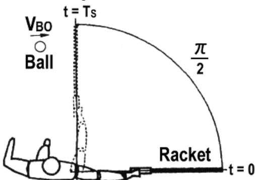
Fig.14 Simple forehand groundstroke swing model.
