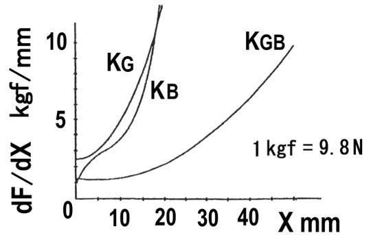
Fig.4 Stiffness vs. deformation of a ball, strings, and a composed ball/string system assuming that a ball deforms only at the side in contact with the strings.
