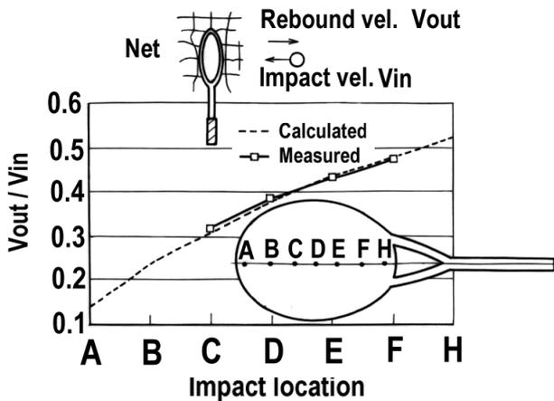
Fig.13 Comparison between the measured rebound power coefficient  $e$  and the predicted one ( $V_B = V_{out}$ ,  $V_{Bo} = V_{in}$ ,  $V_{Ro} = 0$ ).
