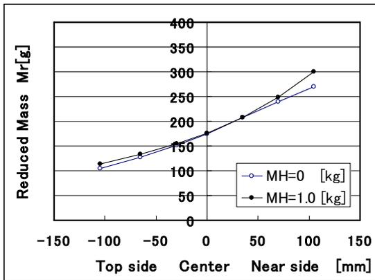
Fig.7. The effect of the arm on the reduced mass of a racket at the impact locations (super-light weighted racket 290 g,  $M_H=1.0$  kg: with arm,  $M_H=0$  kg: without arm)
