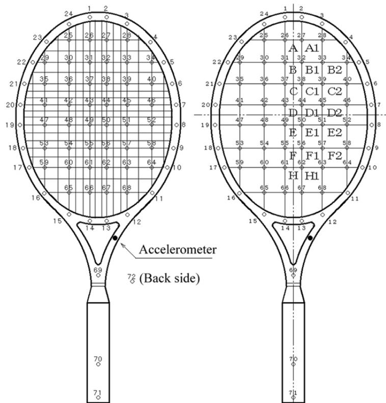
Fig.11 String mesh (Left side) and impact location on the racket face (Right side).
