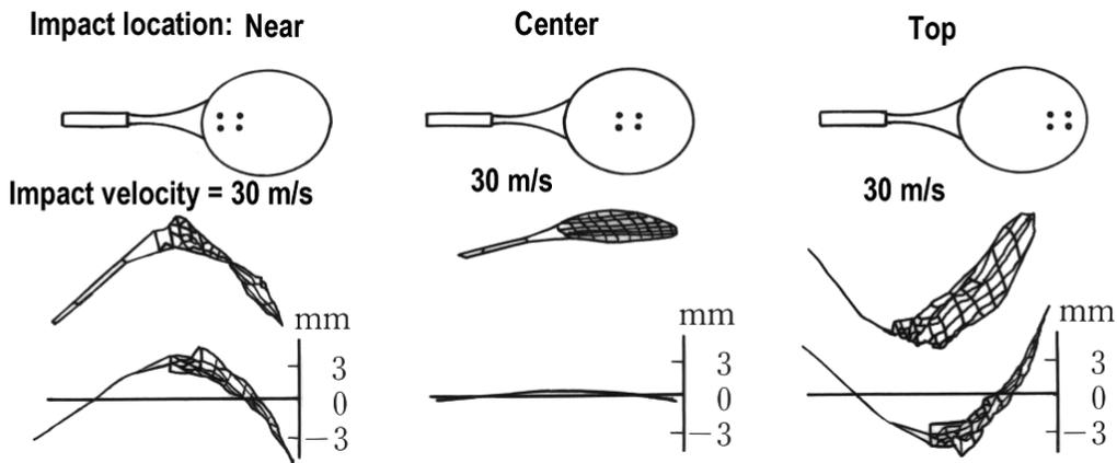
Fig.12 Predicted initial amplitude of 1st mode component of racket frame vibrations.
