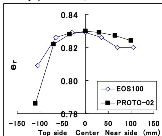
Fig.16 Predicted Restitution coefficient  $e_r$  on the longitudinal axis of racket face when a player hits a ball ( $N_s = 56.9 \text{ Nm}$ ,  $V_{Bo} = 10 \text{ m/s}$ ).
