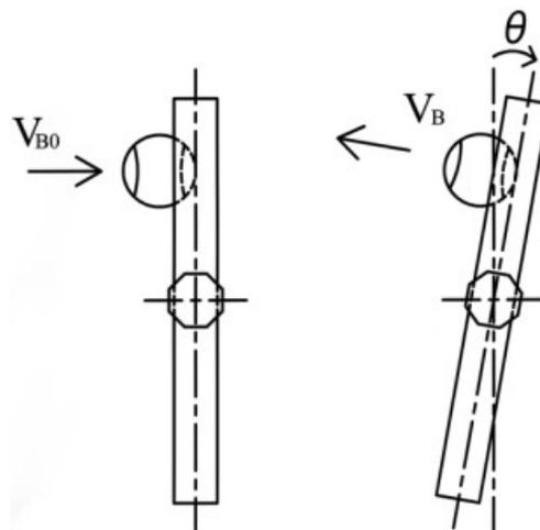
Fig.20 Twist or turn about the long axis when the ball hits the strings at the location away from the long axis of a racket.
