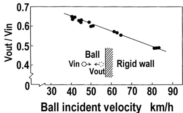
Fig.5 Measured coefficient of restitution (COR) between a ball and a rigid wall.
