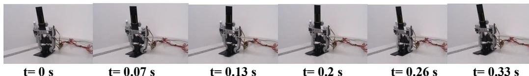
Fig.6 Emergence of simple humanlike robust walking NANBA of biped robot GENBE No.2. Height: 30 cm, walking speed: 10 cm/s (2 km/h: reduced walking speed to height 170 cm)
