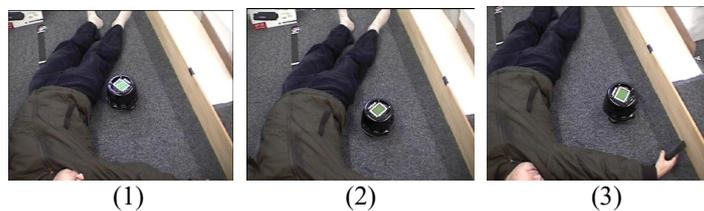
Fig.14 Behaviors of avoiding a moving human body lying down outside experimental environment.
