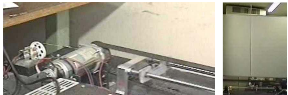
Fig. 4 Stabilizing control of an inverted pendulum on a cart by a computer controller with PID
