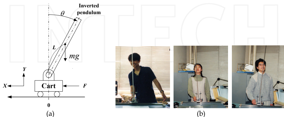
Fig. 1. Stabilizing control of an inverted pendulum.
